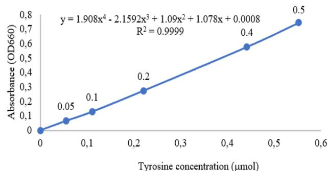
**Figure 4** Standard curve of tyrosine at wavelength 660 nm
