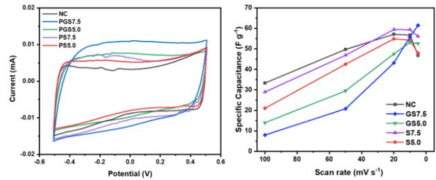
**Figure 2** (a) CV plots at scan rate of 5 mV·s<sup>-1</sup> and (b) specific capacitance value at different scan rate of different MCDI electrodes
