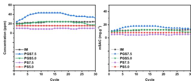
**Figure 5.** (a) Salt concentration and (b) mSAC value of different MCDI electrodes after 30 cycles of CDI process using different MCDI electrodes (Applied voltage:  $1.2\text{ V}$ , flow rate:  $10\text{ mL}\cdot\text{min}^{-1}$ )
