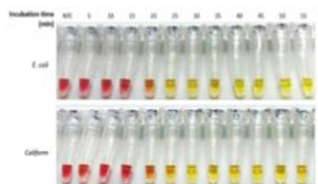
Figure 2. Time optimization for the LAMP assay detecting E. coli and Coliform.
