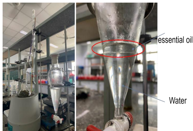
Figure 2. Lemon-scented eucalyptus essential oil distillation system
